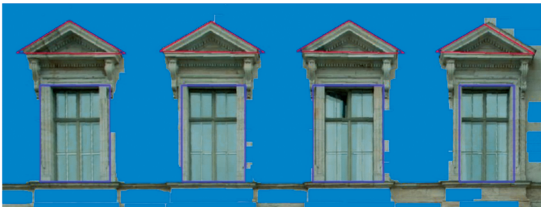
Fig. 2: Segmentation of rectified façade image. We show all pixels which correspond to the façade plane in blue. They are homogeneous with respect to the intensity values. The corresponding 3D points are close to the plane and their variance with respect to the distance is low. In magenta we show the results of window detection and in red the detected triangular cornices.
