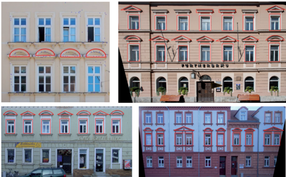
Fig. 6: Results of cornice detection for façades from Freising (top row) and from Schwabach (bottom row) in Germany. All images were manually rectified. The image at top left is limited to the upper floors and shows the detected cornices in red and 3D points in front of the façade in blue. The other three images show the whole façade with detected windows in upper floors and cornices in red. Note that the cornices above the twin windows in the image at bottom right were successfully detected, because the window detection returned one window instead of two.
