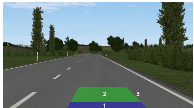
Figure 1: The Predictive Corridor (PC) shown during the user study. It displays the predicted position (1) of the remote Autonomous Vehicle (AV) and the path of the full braking (2). The width of the PC (3) corresponds to that of the AV.
