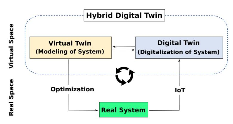
In light of the increasing digitalization of our world, digital twins have great potential to contribute to protecting and maintaining critical infrastructures. In case of bridges, digital twins can have a crucial role in structural health monitoring (SHM) [1].
