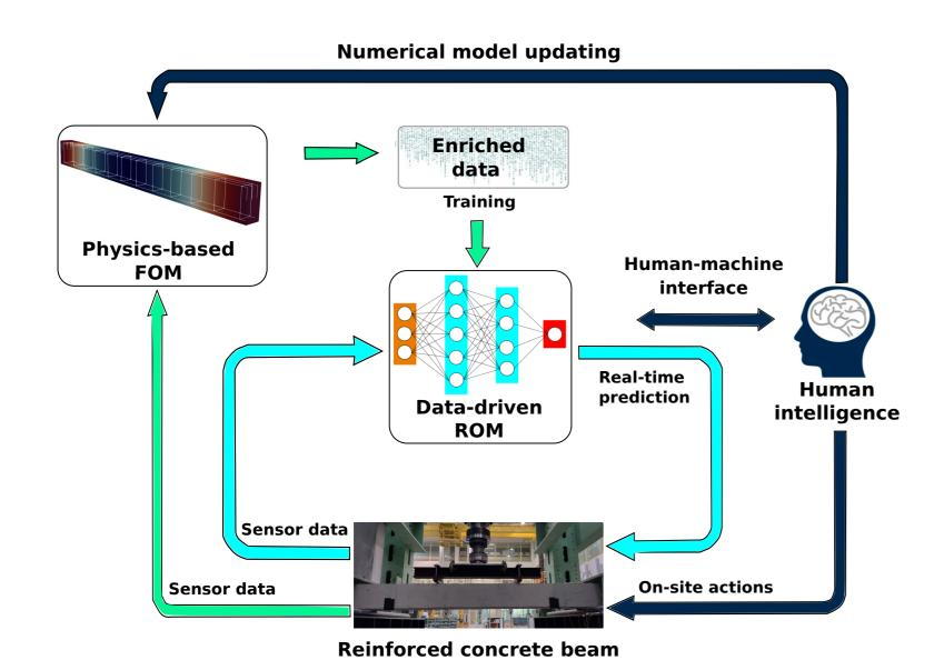
We combine a physics-based full-order model (FOM) with a fast-to-evaluate data-driven reduced-order model (ROM) interacting with sensor data of the physical asset. The full-order model provides a detailed understanding of the physical behavior and is employed to calibrate the reduced-order model aiming at a reliable digital representation. The combined model has the following capabilities:
