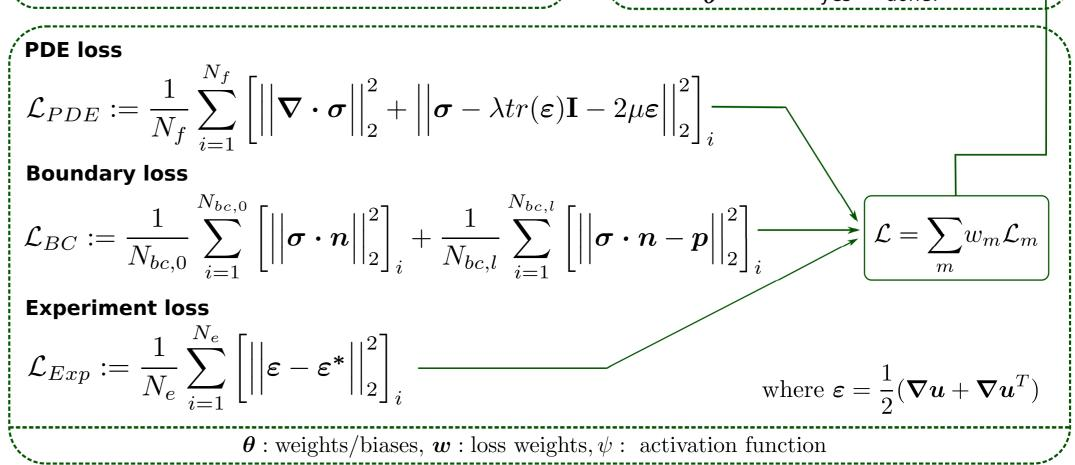
The data-driven ROM is based on **p**hysics-**i**nformed **n**eural **n**etworks (PINNs) that combine differential equations and measurement data in the loss function of neural networks [3].
