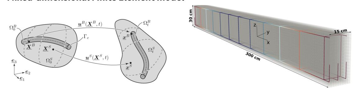
The physics-based FOM is based on a novel finite element formulation with beam-to-solid mesh tying. We use this method to capture the interaction between the reinforcement components and the concrete matrix of the beam [2].
