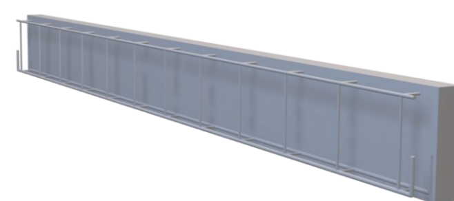
Figure 6 – Modified 3D model of steel-reinforced concrete beam
