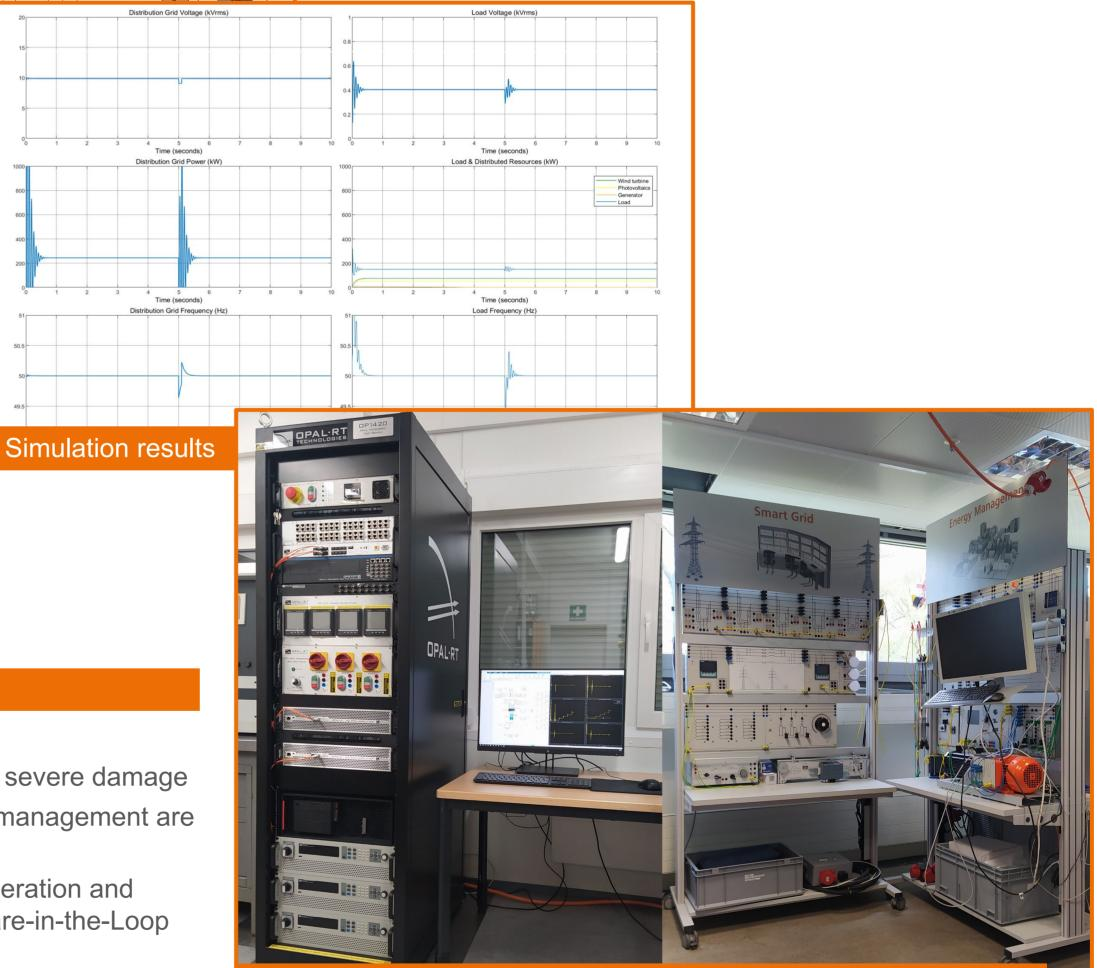
Further simulative investigations of electrical faults and emergency operation and validation with real-time testing of components using a Power-Hardware-in-the-Loop (PHIL) test bench
