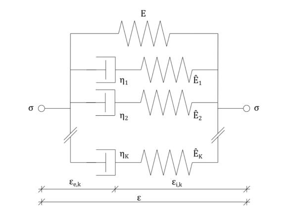
Elastic response: Hyperelastic springs – Cauchy stress according to Yeoh model
