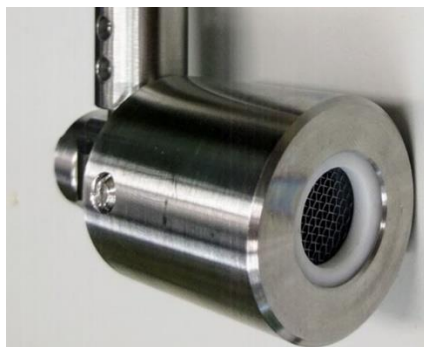
a) Figure 7. Retarding potential analyser. General view (a) and electrical scheme (b).
