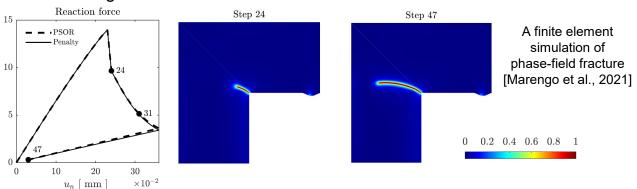
In this thesis, we focus on the phase-field model for brittle fracture in a dynamic framework investigating the role of explicit time integration schemes (e.g., Newmark, 1959). Numerical simulations will be carried out using an in-house finite element code.
