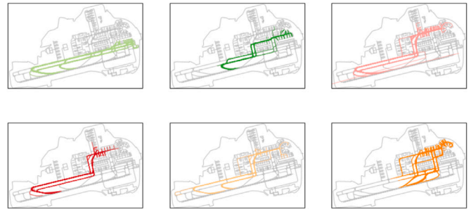
Fig. 12. Cluster subset based on three features (latitude, longitude and ground speed) and 50 samples per trajectory. The top right (pink) and bottom left (red) correspond to similar spatial flows but different ground speed profiles (see Fig. 13). (For interpretation of the references to color in this figure legend, the reader is referred to the web version of this article.)
