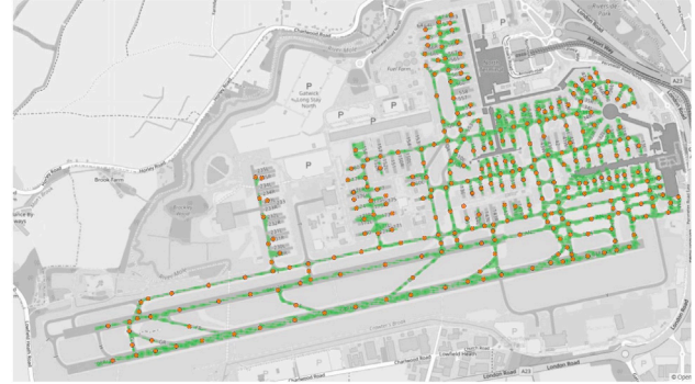
Fig. 5. Density-based clustering of transmitted aircraft positions to derive airport infrastructure, such as parking positions or operational network (e.g. taxi way connections) validated against information from OpenStreetMap.
