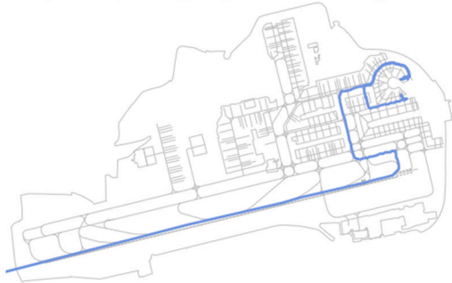
Fig. 7. Invalid aircraft ground trajectories detected in the dataset of London-Gatwick Airport.
