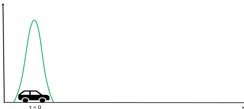
Figure 3.1: Determining the position of a vehicle (one Gauss distribution)
