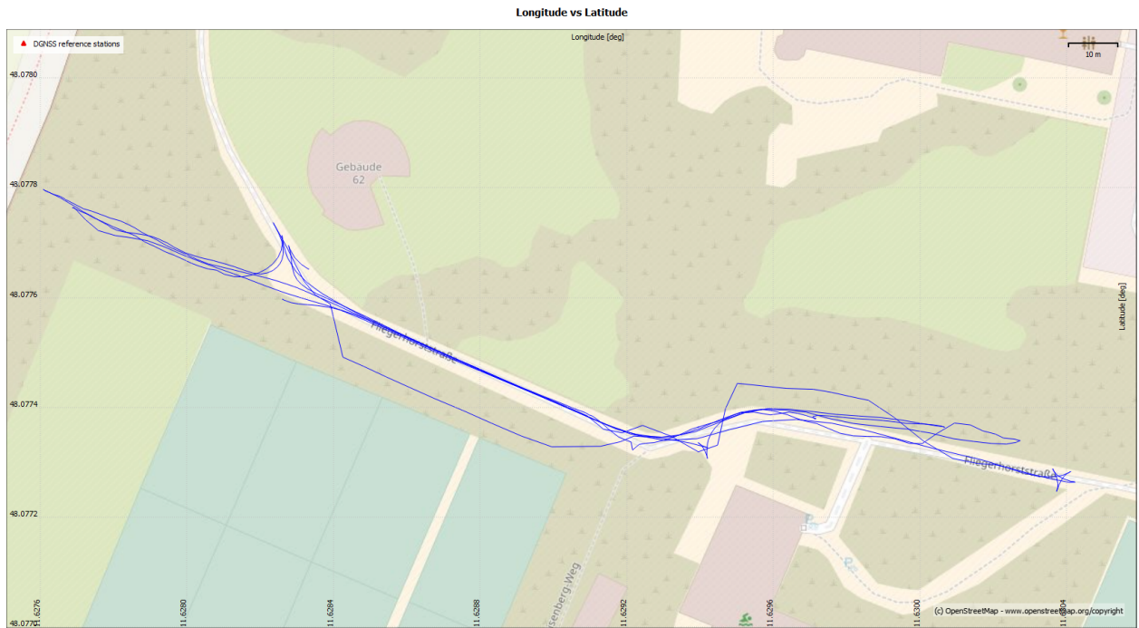
Figure 6.26: Driveway of the measurement bus with GNSS only solution
