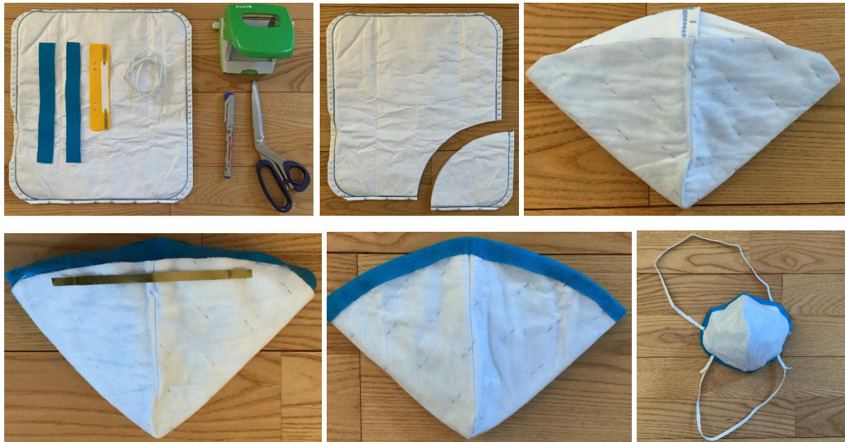
Materials required to manufacture a mask and the different manufacturing stages from top left to bottom right
